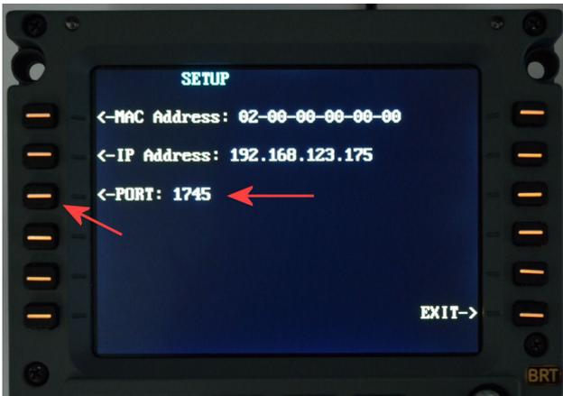
If required by avionics software, set also the communication port by typing it from keyboard and by pressing LSK-3 instead. 1745 is the Default useb by Prosim and PMDG, but You can change it for specific purposes.
