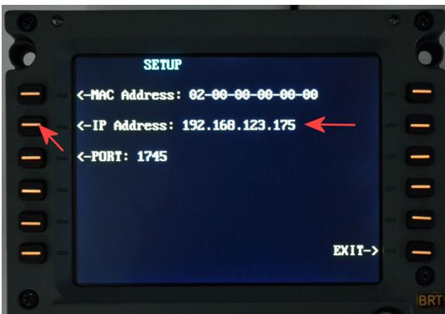
After a few seconds, the "SETUP" screen on the left will be displayed, if not, unplug the power cable and repeat.
