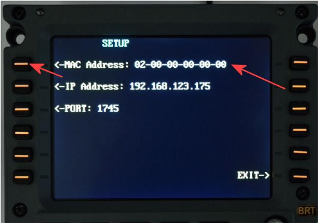
In the same way, using the FMC keyboard, change the MAC address, by adding a single number:02-00-00-00-01 should be good, because in a networked multi CDU system the mac address of every CDU must be unique, confirm with LSK-1. Please note: the first number of Mac address must remain "02".
